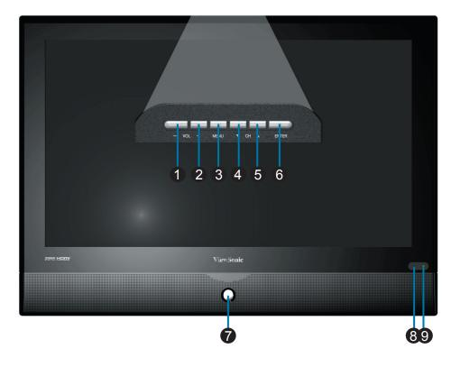
Volume Down Decrease sound volume or adjust a highlighted control while in OSD menu. 2 Volume Up Increase sound volume or adjust a highlighted control while in OSD menu. 3 Menu Turn OSD menu ON/OFF. **4** CH Down Channel down when source is TV, or select a control while in OSD menu. **5** CH Up Channel up when source is TV, or select a control while in OSD menu. 6 ENTER To highlight a control in OSD menu. Power ON/OFF button 8 Remote Control Receiver Power LED Indicator
