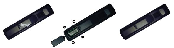
1 Remove the battery cover by pulling then lifting the knob on the cover.
