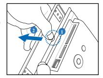
3. To install a new front panel, align the panel edge to the Digital Photo Frame and gently place the panel on the device.
