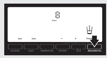
Press ICE MODE to manually turn off the Measured Fill feature.
