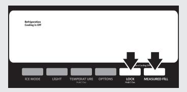
• Press and hold LOCK and MEASURED FILL together for 3 seconds again to turn cooling back on.
