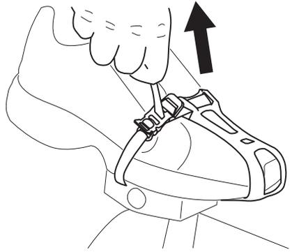
To remove your foot from the toe clip, push on the plastic tab to loosen the strap.
