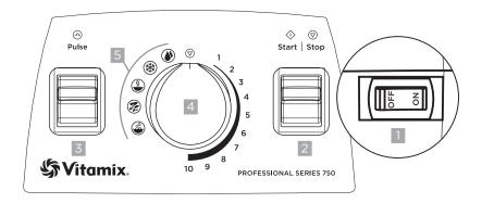
On / Off Switch: The On / Off (or Power) Switch is located on the lower right-hand side of the machine. The On / Off Switch controls the power to the machine.
