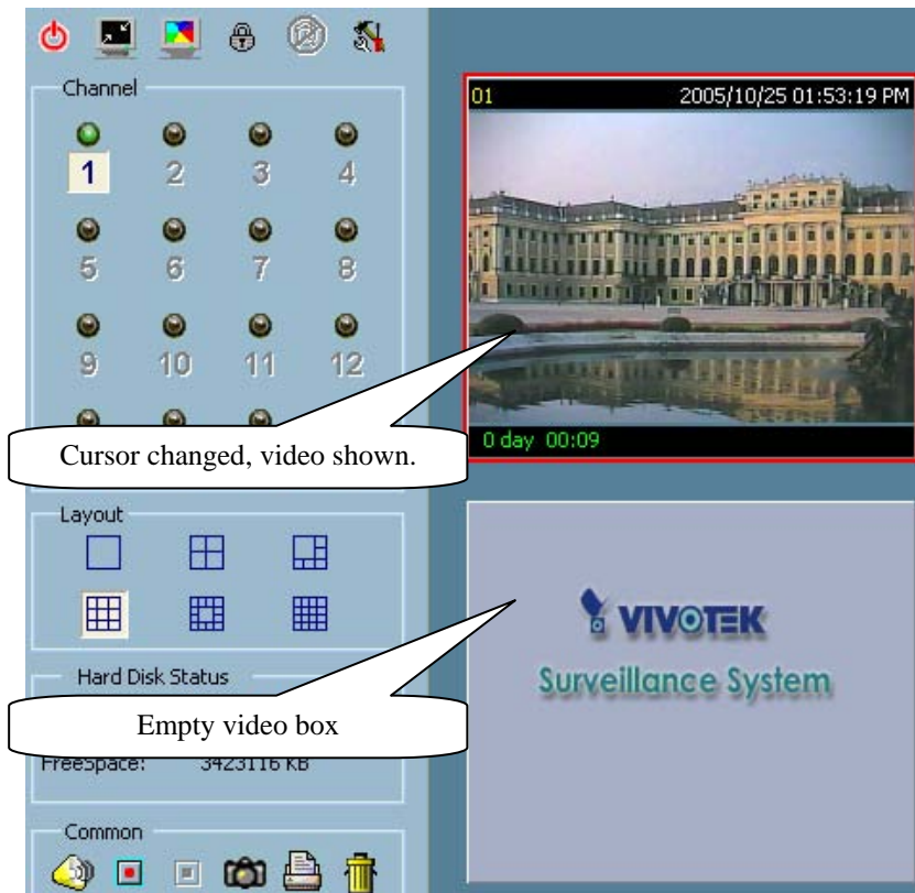
Figure 3-26 Showing Video on the Displaying Frame
