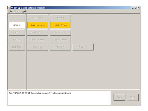
NX-100 units that are not connected are displayed in the message display area. Depending on the displayed messages, perform operation again after temporarily terminating the program and waiting a short time, or after correcting any setting- or unit-related problems. The Selection buttons change to orange if a connection is made to at least one of the NX-100 units programmed for that button.
