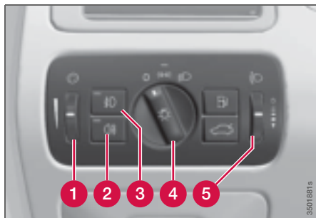
Overview, light switches
