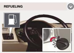
Press this button to unlock the fuel filler door. Recommended octane rating: 91 Minimum octane rating: 87
