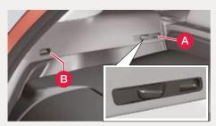
Place one rear lock at (B) and press the lock button forward. Lock the other buttons in the same way.
