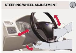
Adjust tilt and telescope. WARNING! Never adjust the steering wheel while driving.
