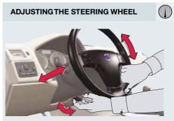
WARNING! Adjust the steering wheel before setting off, never while driving.
