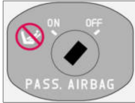
Switch for SRS in OFF position.
