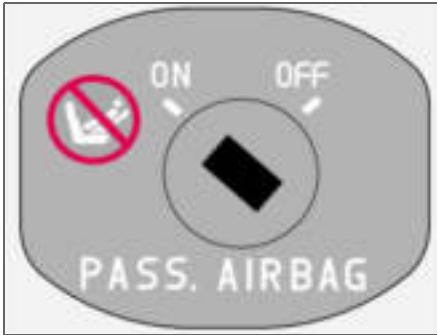
Switch for SRS in ON position.
