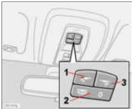
Passenger compartment lighting and reading lamps.
