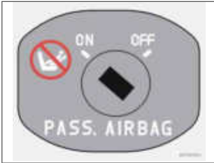
Switch for SRS in ON position.
