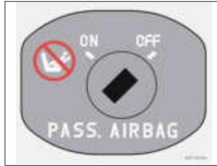
Switch for SRS in OFF position.
