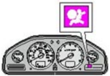
SRS warning light
