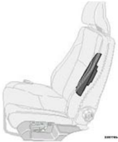
Location of the side impact (SIPS) airbag
