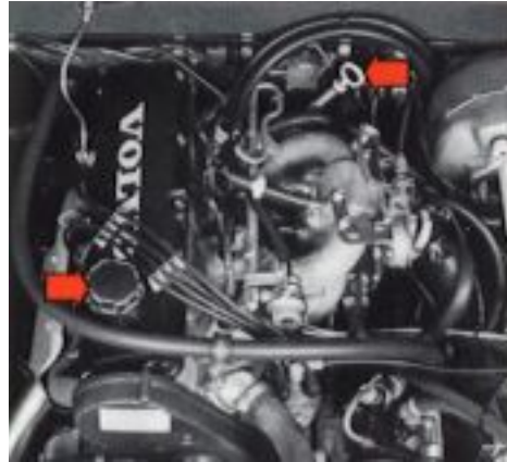
Checking oil level
