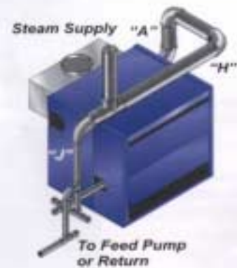
Recommended Minimum Pipe Sizes For Dual Risers
