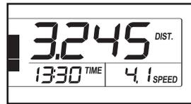
time you change the incline, the display will show the incline setting for a few seconds. Note: When a program is selected, the display will show the time remaining in the program instead of the elapsed time. When a distance goal program is selected, the display will show the number of kilometers remaining in the program instead of the distance that you have walked or run.
