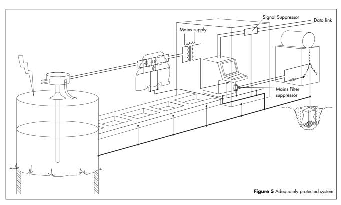
supply will contain a significant amount of surges but if for any reason the supply is particularly exposed to invasion from lightning induced surges then some consideration to suppressing the main supply should be given.
