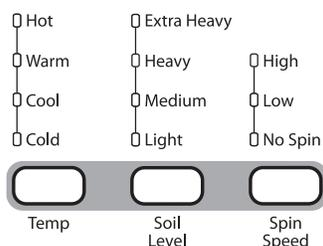
Once you select a cycle, the default settings for that cycle will be lit. Press the cycle settings buttons to change the Temperature, Soil Level, and Spin Speed, if desired.
