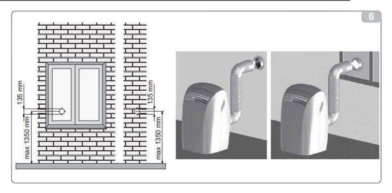
When you use this air conditioner unit, hot air must be exhausted out of the room to complete the air exchange of the condenser. When the unit is operating in fan-only mode, no exhaust is required.
