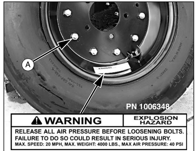
Figure 9. Split Rim Tire Servicing
