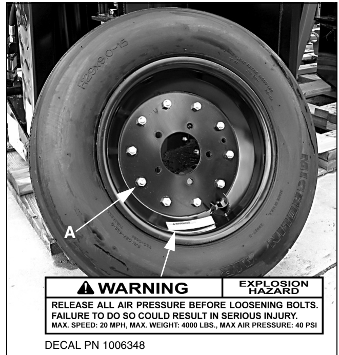
Figure 19. Split Rim Tire Servicing
