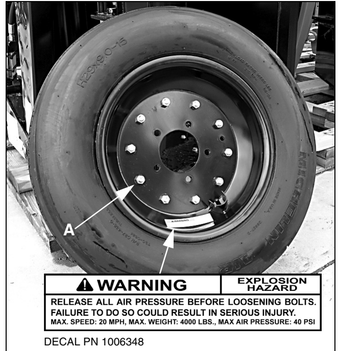
Figure 10. Split Rim Tire Servicing
