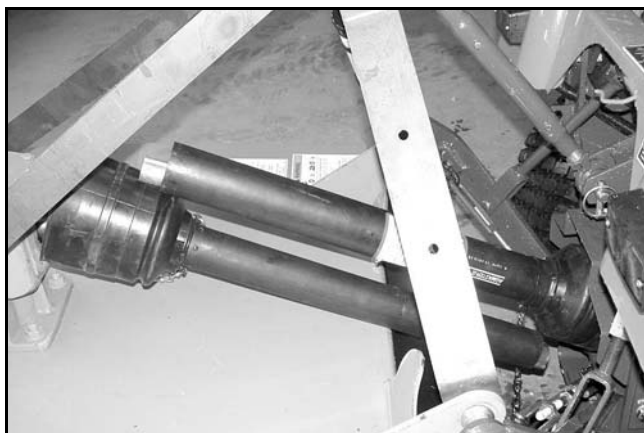
Figure 4. Drive Halves Placed Parallel
