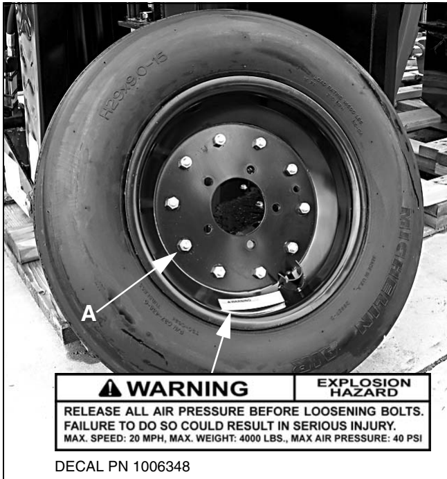
Figure 15. Split Rim Tire Servicing
