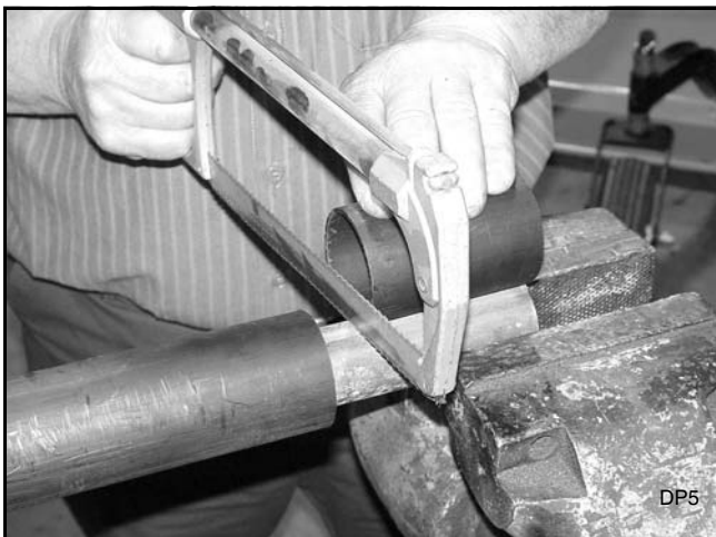
Figure 7. Cut Shaft to Length
