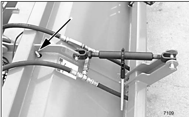
Figure 24. Gearbox Oil Fill Location
