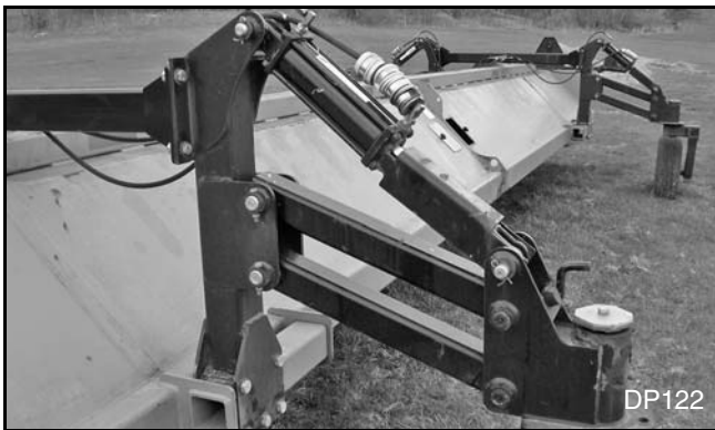
Figure 42. Pivot Tubes, Caster Pivots & Cylinders Installed
