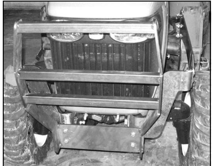
Figure 8. Grill Guard Installed
