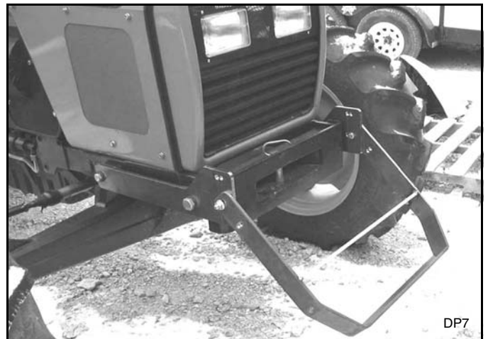
Figure 9. Grill Guard Installed (Typical)
