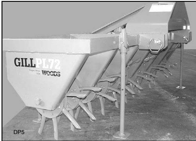
Figure 6. Parking Stands Lowered into Storage Position
