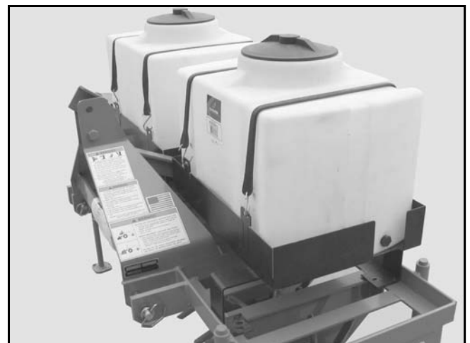
Figure 8. Water Tanks Installed
