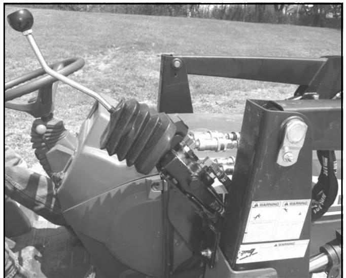
Figure 14. Single-Lever Control Valve
