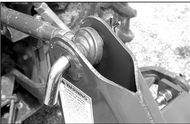
Figure 3. Top Link Connected - Rear Blade
