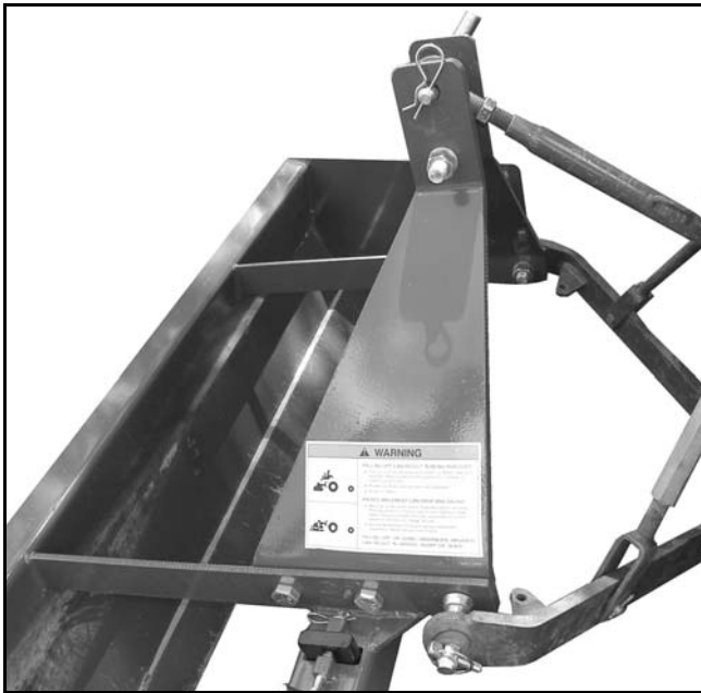
Figure 2. Top Link Connected - Box Scraper
