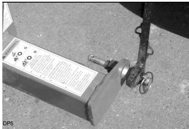
Figure 1. Lower Lift Arm Attachment, Category 1
