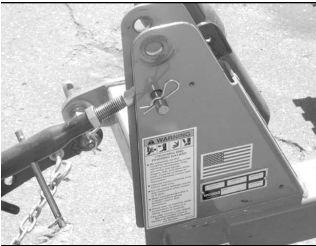
Figure 4. Top Link Connection
