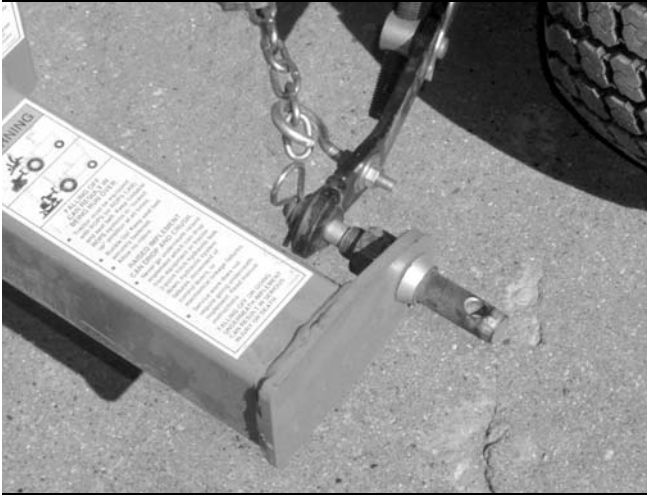
Figure 3. Lower Lift Arm Attachment, Category 0
