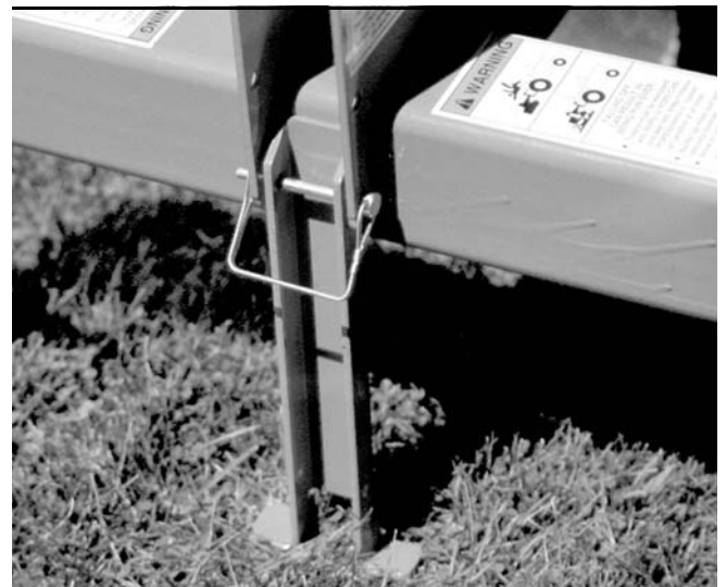
Figure 8. Parking Stand - Storage Position
