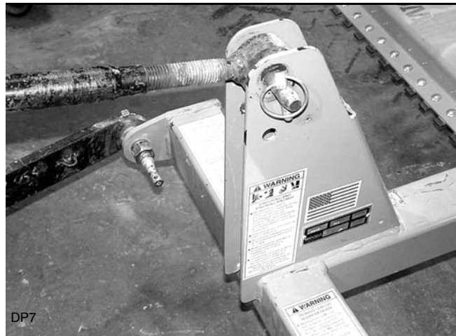
Figure 2. Top Link Connection
