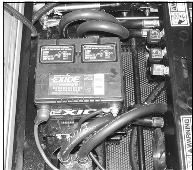
Figure 8. Battery Located Under Seat
