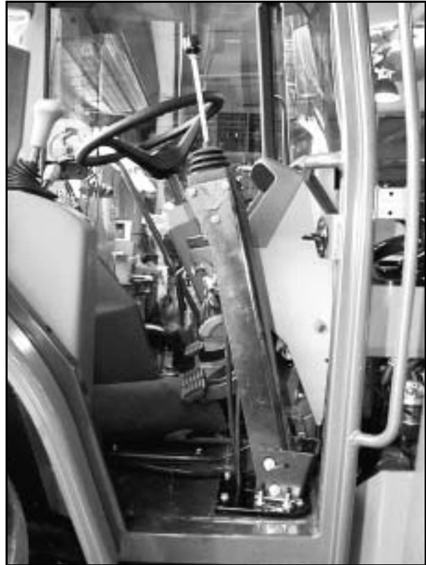
Figure 28 Controller Stand Installed
