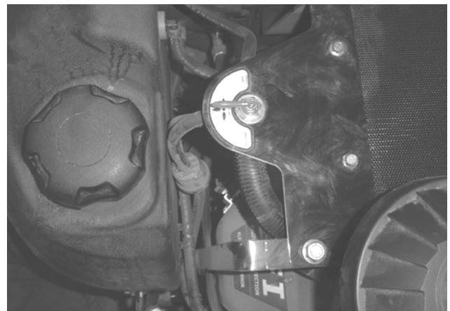
Left Tank: Fuel flows from the left tank when the selector is turned 1/4 turn toward the left hand side of the machine.
