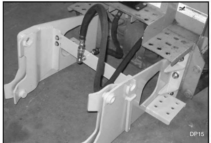
Figure 29. Backhoe Hose Connection, Storage Position (Typical)
