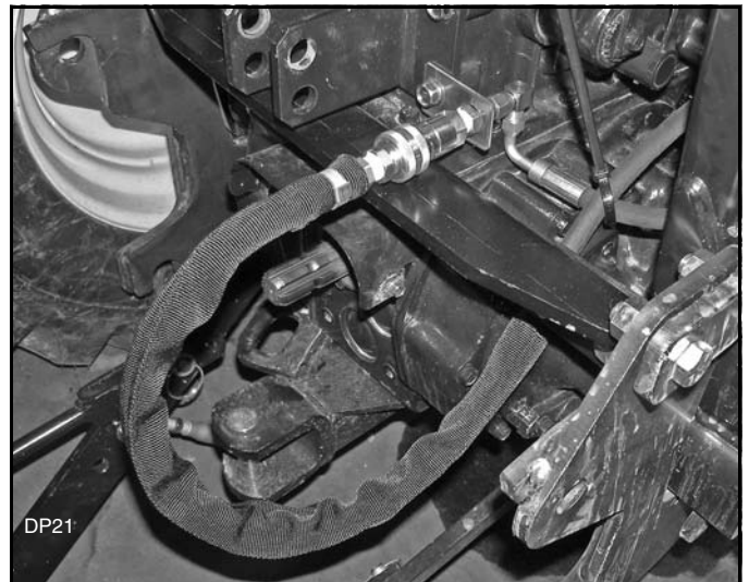
Figure 28. Hose Connection - Backhoe Removed
