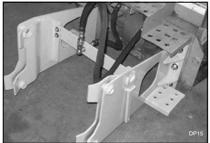
Figure 29. Backhoe Hose Connection, Storage Position (Typical)
