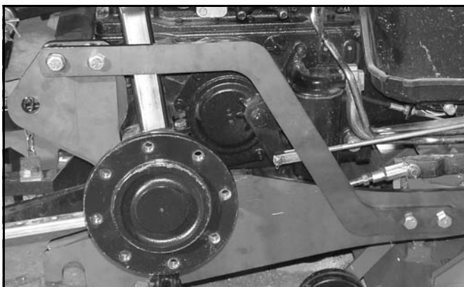
Figure 13. Offset Bar Installed, Right Side
