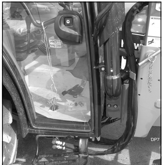
Figure 10. Hydraulic Hose Connection
