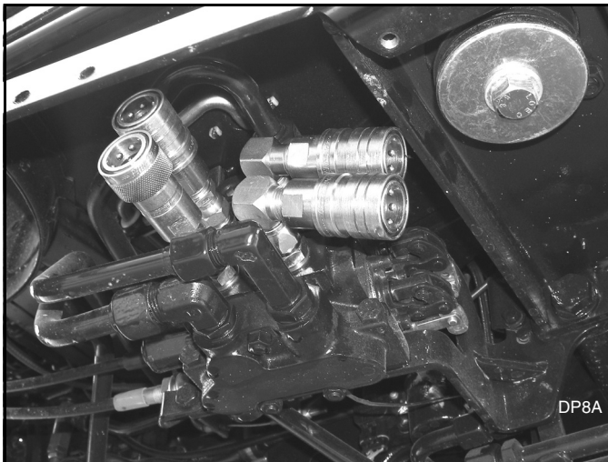
Figure 11. Hydraulic Fitting Installed, Bottom View
