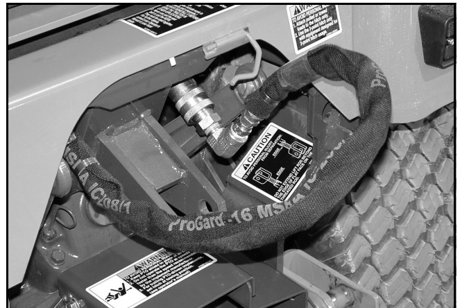
Figure 13. Hose Connection - Backhoe Removed
