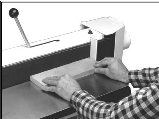
Figure 47. ALWAYS use the back stop, and keep your fingers away from the belt.
