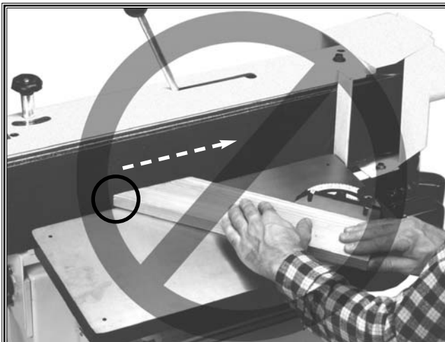
Figure 5. DO NOT sand wood with sharp corners at the leading-edge of the sanding operation. The belt can grab and throw the wood.
