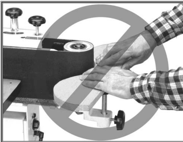
Figure 3. DO NOT sand wood with your fingers close to the idler roller and belt.
