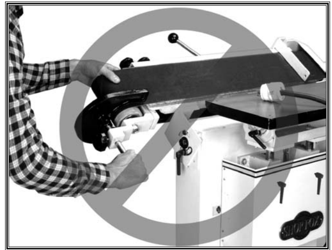
Figure 43. Incorrectly holding and tilting the platen.
