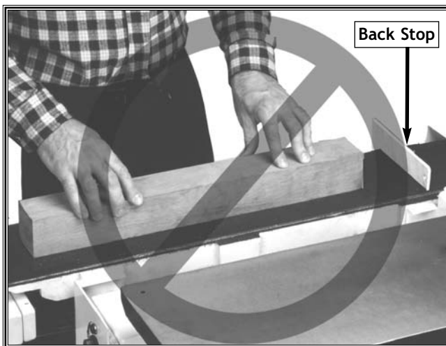
Figure 51. Incorrect face sanding away from back stop.
