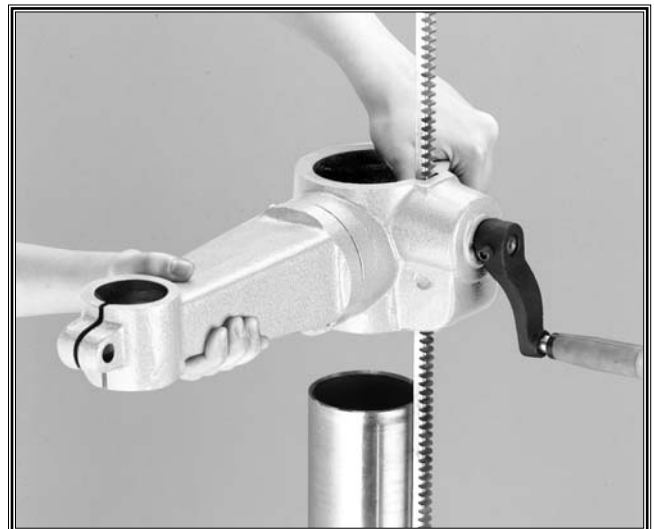
Figure 11. Correct rack orientation.
