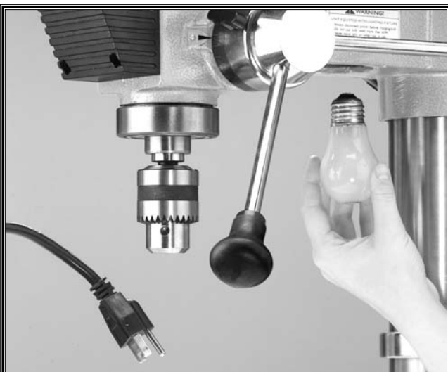
Figure 17b. Installing a light bulb.
