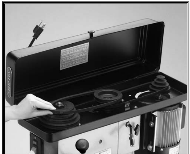
Figure 24. Adjusting belt to desired speed.
