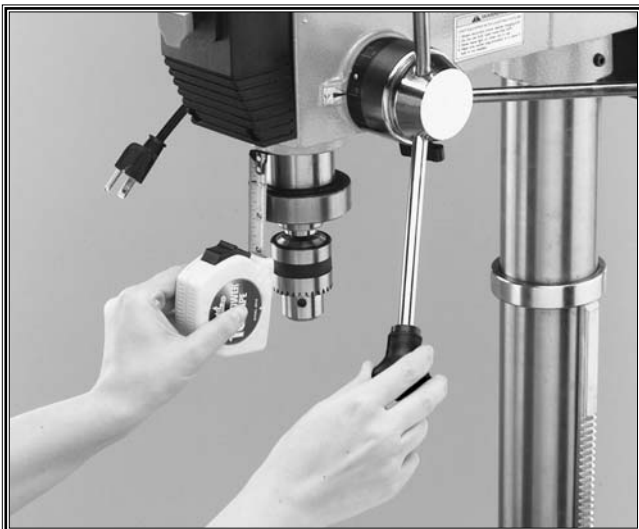
Figure 27. Actual stop depth being measured.
