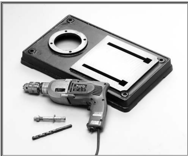
Figure 7. Secure base to floor.
