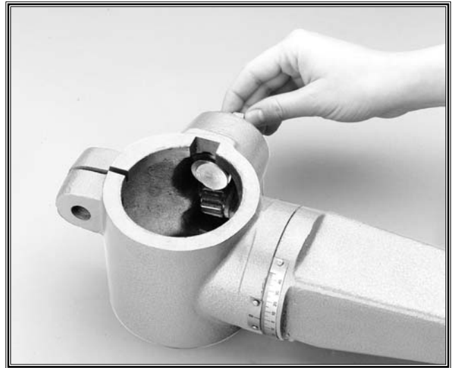
Figure 9. Insert the pinion gear from the inside.
