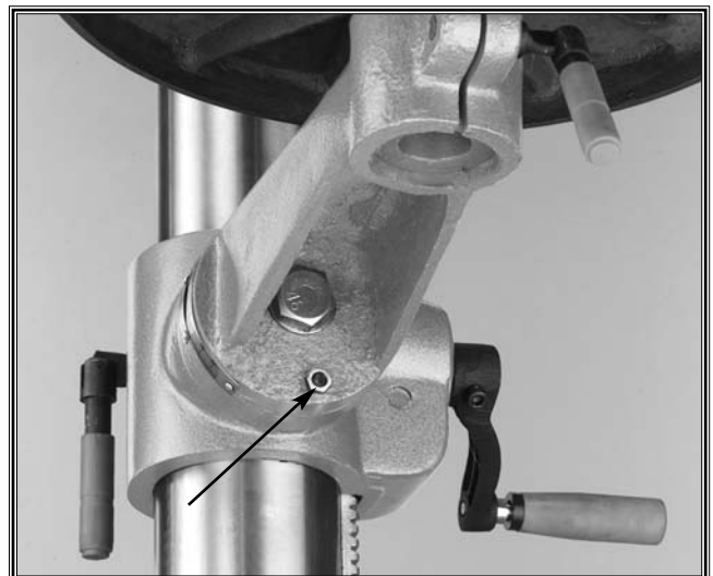
Figure 30. Locating pin and nut.
