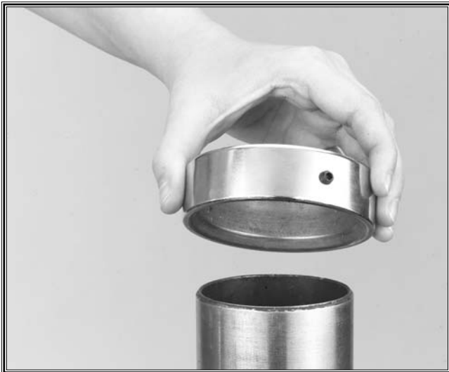
Figure 13. Inside bevel in the correct position.
