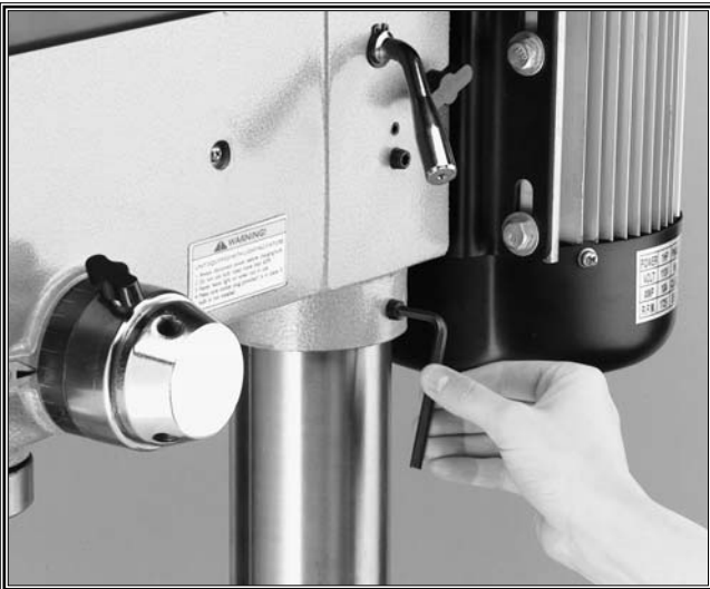
Figure 16. Tighten setscrews to secure headstock.
