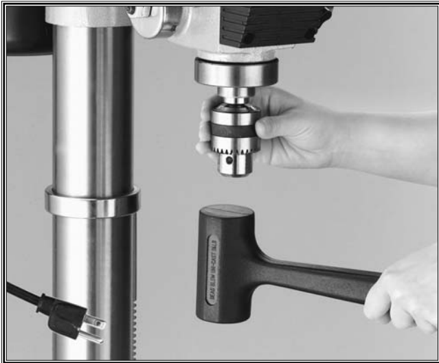
Figure 20. Seating arbor into spindle.
