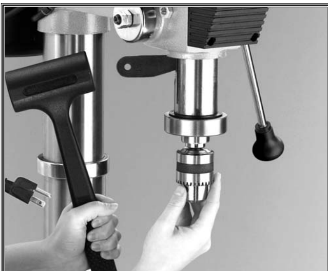
Figure 22. Using wedge to remove arbor.
