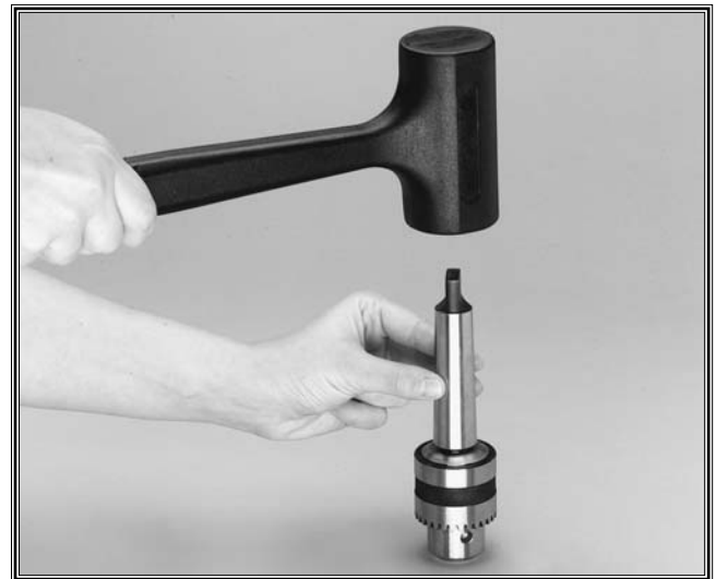
Figure 19. Seating the arbor into chuck.
