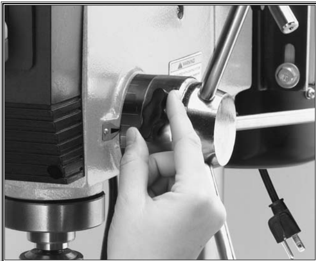
Figure 26. Loosening collar lock knob.
