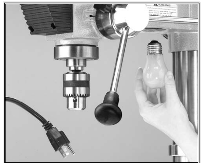
Figure 5. Unplug machine when changing bulbs.
