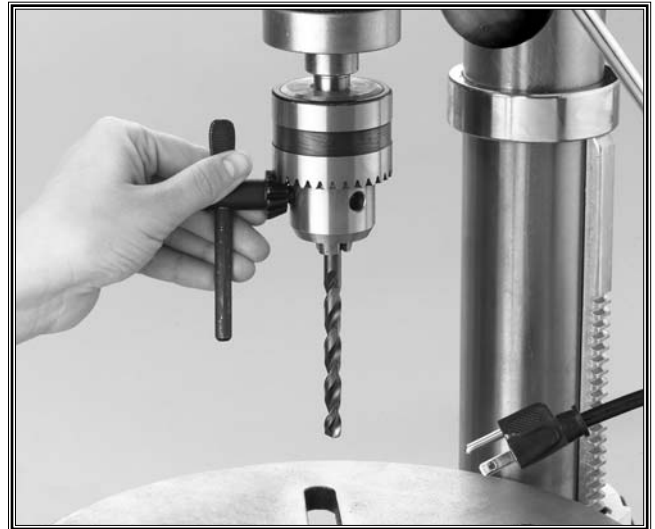
Figure 33. Chuck key engaged.
