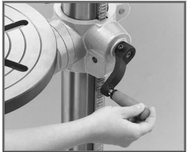
Figure 28. Changing table height with crank.
