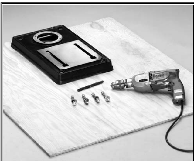
Figure 8. Secure base to plywood.
