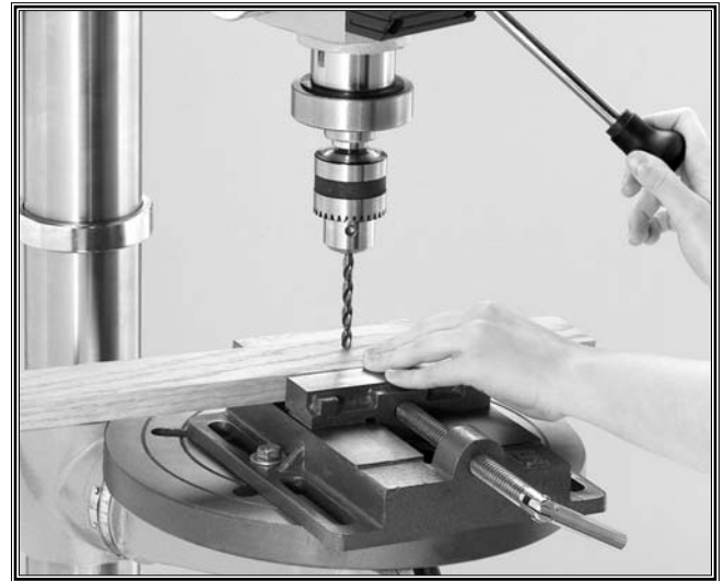
Figure 3. Keep fingers away from spinning tool.
