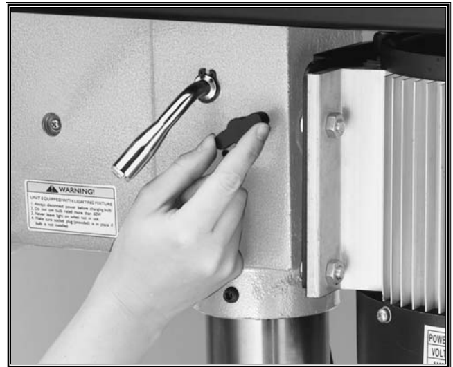
Figure 23. Loosening the lock knob.
