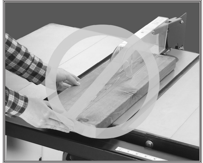
Figure 5. Do not freehand cuts.
