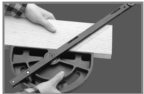
Figure 44. Using the miter gauge to mark the angle of a miter cut.
