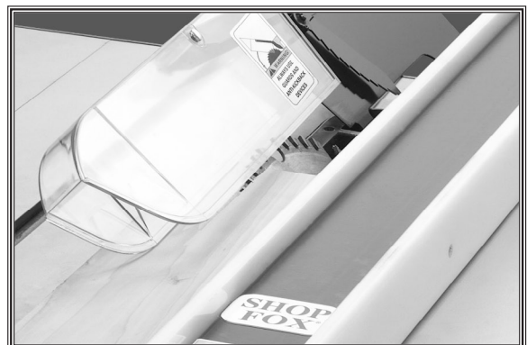
Figure 42. Typical 45^\circ rip cut.
