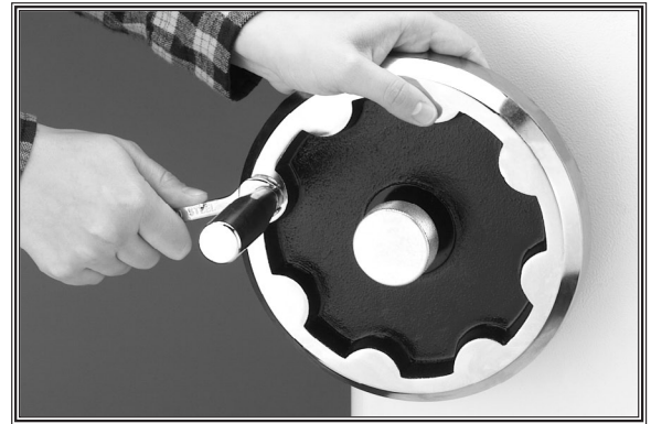
Figure 22. Installing handwheel, lock knob and handle.
