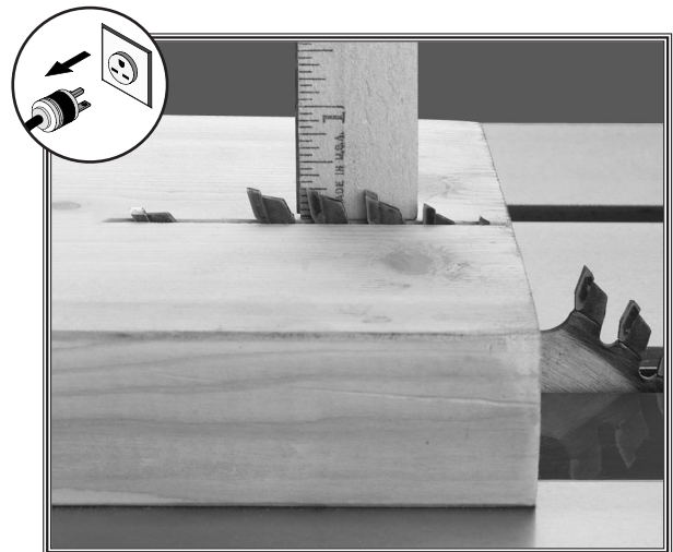
Figure 32. Top of blade protruding approximately \frac{1}{4} " from workpiece.
