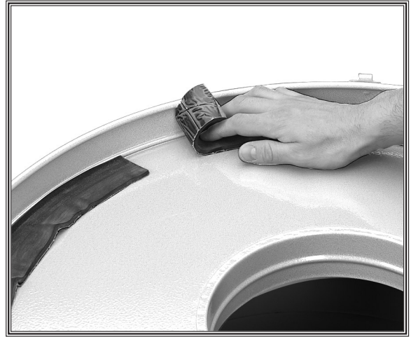
Figure 29. Attaching foam tape to collector drum lid.
