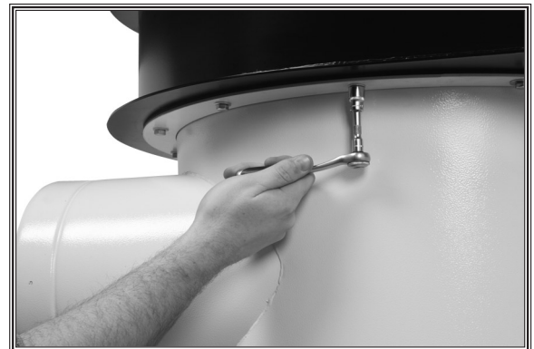
Figure 21. Securing intake barrel to blower.
