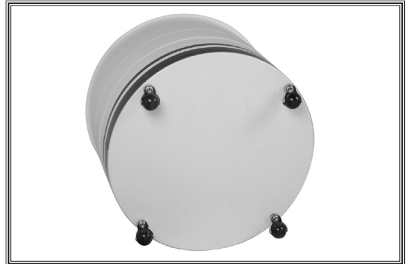
Figure 30. Casters attached to the lower collection drum.
