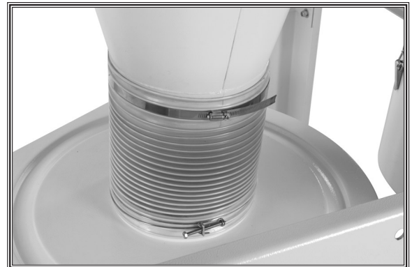
Figure 36. Drum attached to cyclone funnel with 9" hose clamps.
