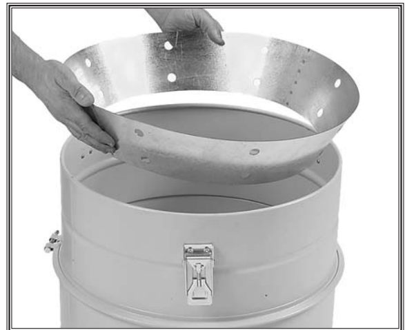
Figure 26. Inserting the collection drum vacuum plate.
