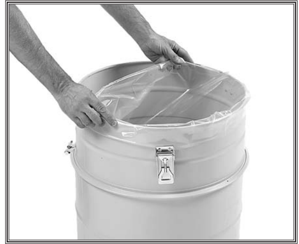
Figure 27. Inserting the plastic collection bag.
