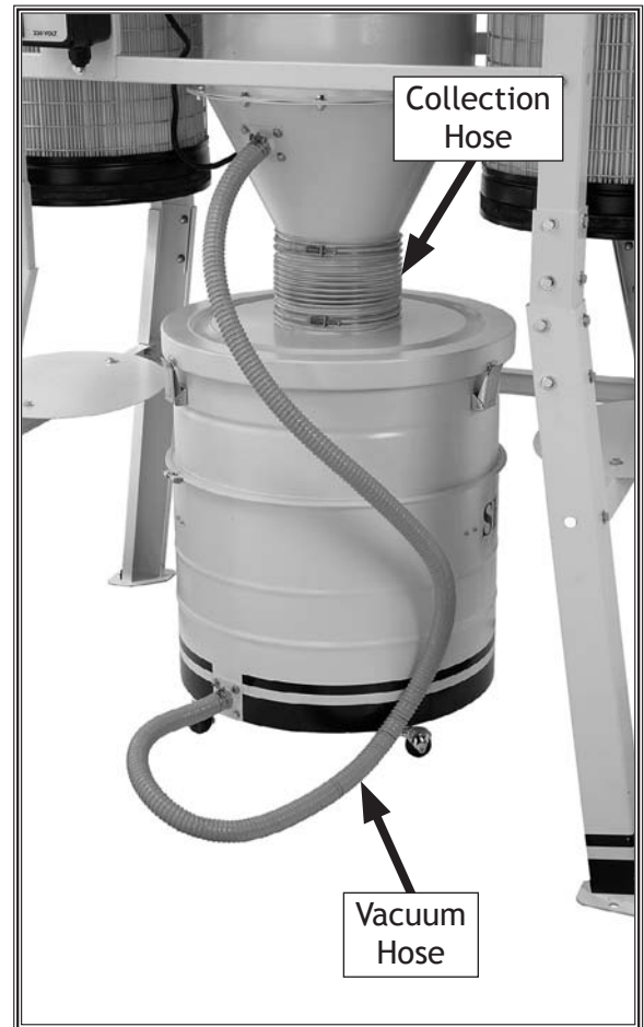
Figure 29. Collection and vacuum hoses installed.
