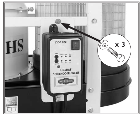
Figure 14. Remote magnetic switch attached.
