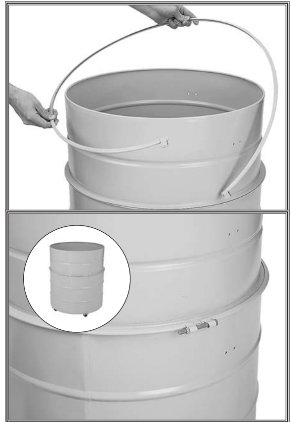
Figure 22. Clamping the top and bottom collection drums together.
