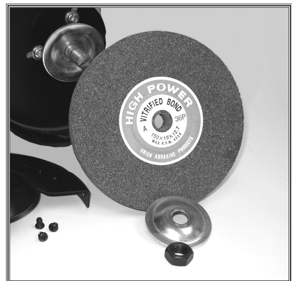
Figure 7. Grinding wheel installation order.
