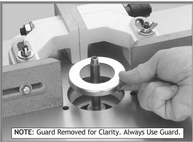
Figure 3. Use the smallest insert the cutter will allow to keep woodchips away from the inside of shaper.
