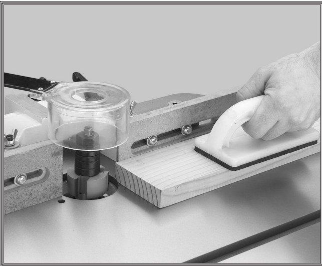
Figure 2. Use rubberized SHOP FOX® Push Blocks to grip the workpiece when cutting.
