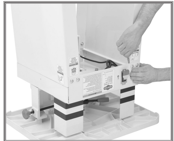
Figure 10. Attaching stand to shaper unit.
