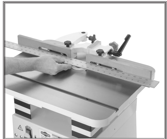
Figure 19. Use straightedge to check fence.
