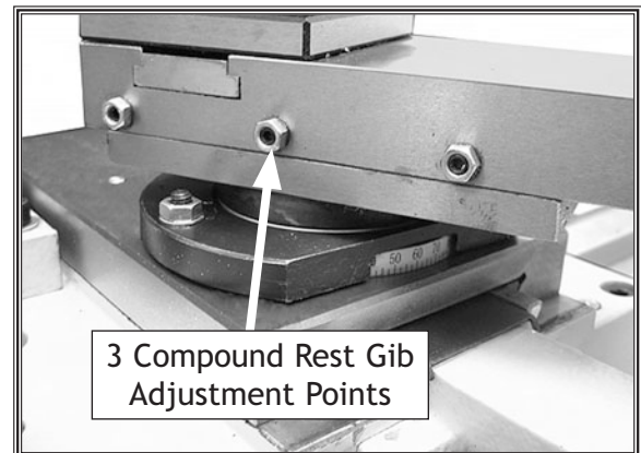
Figure 44. Gib adjustment points.
