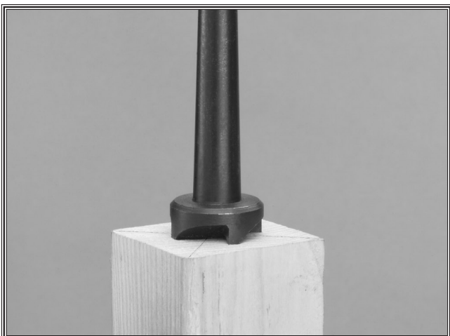
Figure 25. Spur center properly embedded into workpiece.
