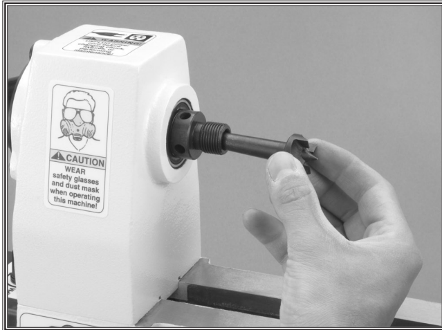
Figure 9. Installing spur center into headstock spindle.
