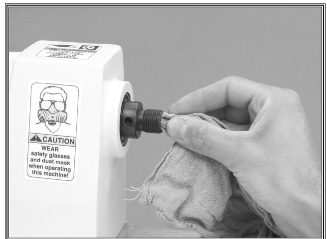
Figure 32. Cleaning spindle tapers.
