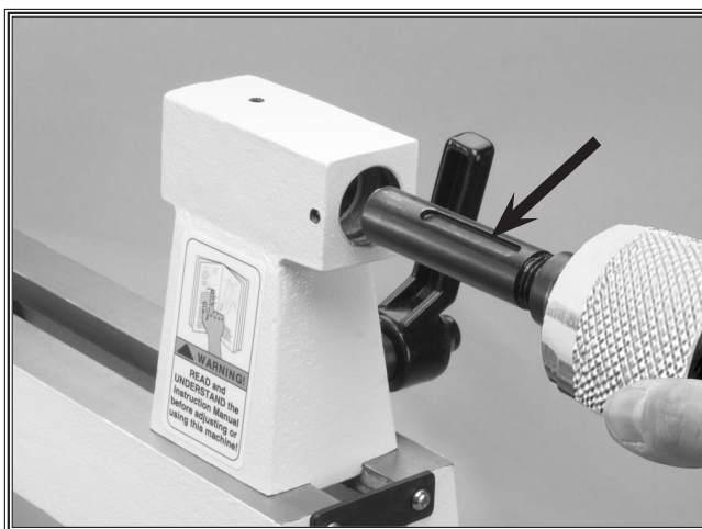
Figure 14. Tailstock barrel alignment slot.
