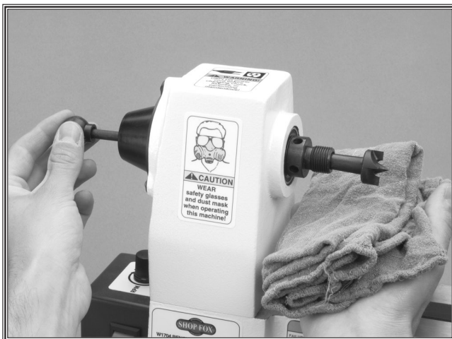
Figure 10. Removing spur center with knock-out tool.
