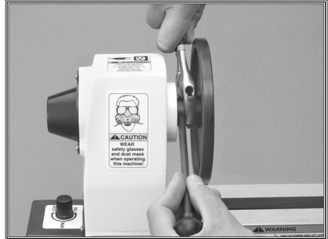
Figure 11. Tightening face plate to headstock spindle.
