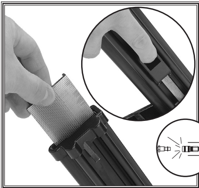
Figure 2. Loading nails into the nailer.
