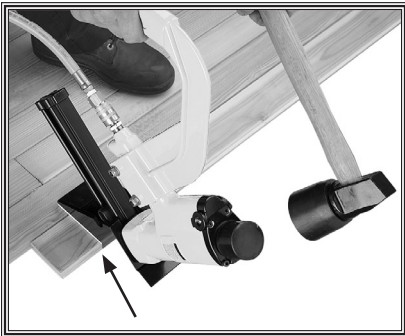
Figure 3. Positioning nailer on flooring strip and operating.
