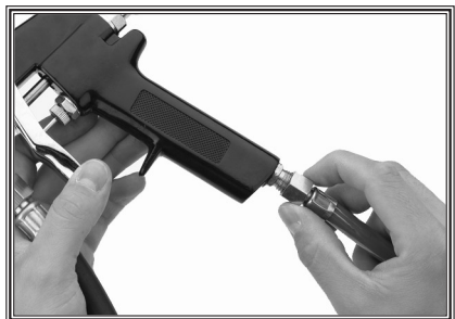
Figure 6. Attaching hose to spray gun.
