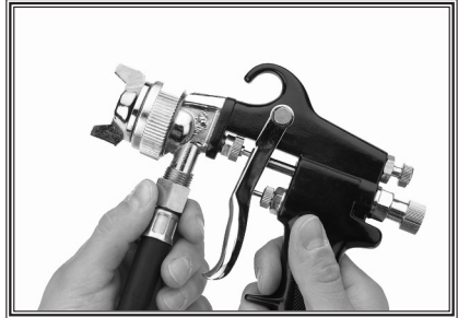
Figure 4. Attaching fluid hose to spray gun.
