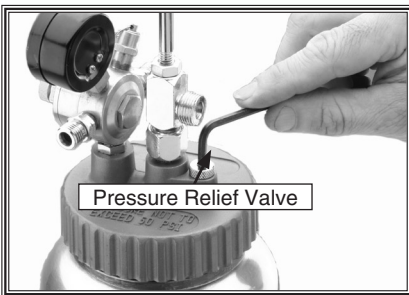
Figure 16. Pressure relief valve.
