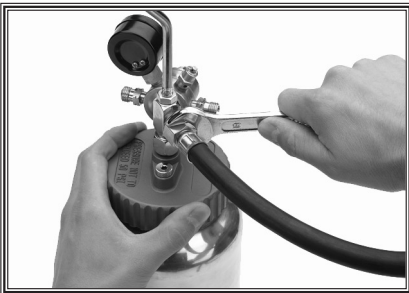
Figure 3. Installing fluid hose.
