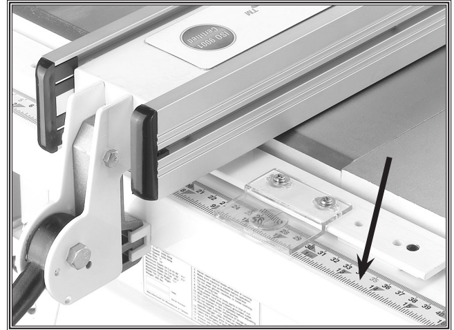
Figure 15. Scale installed on front rail.
