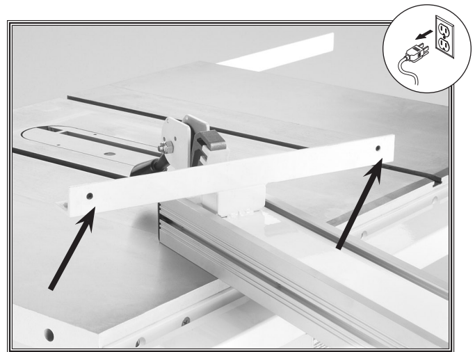
Figure 13. Fence adjustment setscrews.
